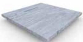
**Mipolam ROBUST EL7** is a dissipative flexible homogeneous vinyl floorcovering available in both sheet and tile. Calendered and compacted. It has permanent antistatic properties ( $< 100$  V). It acts as a continuous dissipater  $10^6 < Rt < 10^8$  (EN 1081) and complies with EN 649.
