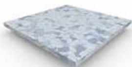
**MIPOLAM TECHNIC EL5** is a conductive flexible homogeneous compacted vinyl floorcovering available in tiles. The conductive carbon coated PVC pellets create a perfect conductive network for permanent conductive properties and antistatic properties ( $< 20$  V) throughout its full life expectancy. It acts as a continuous conductive  $10^4 \leq Rt \leq 10^6$  (EN 1081) and complies with EN 649.
